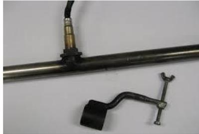
If mounting in the exhaust directly, then keep the sensor close to vertical (or worst case away from horizontal by at least 10°) to keep condensation from entering the sensor e.g. 90°-10° is acceptable range.
