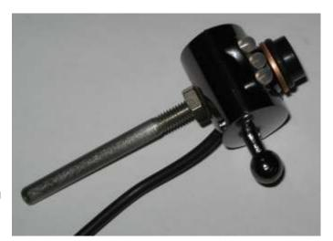
We needed to add a small washer between the lens and the body as when it was screwed out it ended up a bit loose - the washer allows it to be tightened at the focal length you want.
