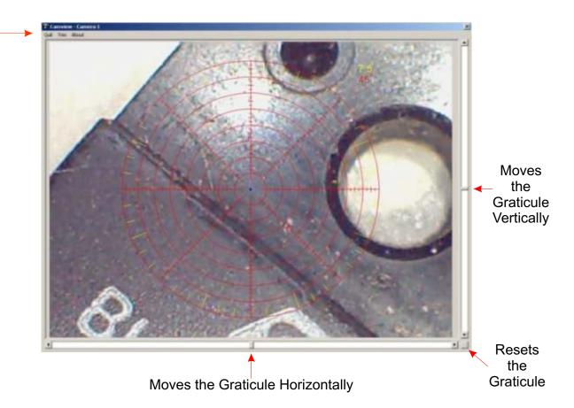
The Horizontal and Vertical Scroll Bars allow the on screen graticule to be moved as required. The changes made using these scrollbars are not saved when CamView is closed. Use the Trim Menu to make permanent changes to Graticule position.
