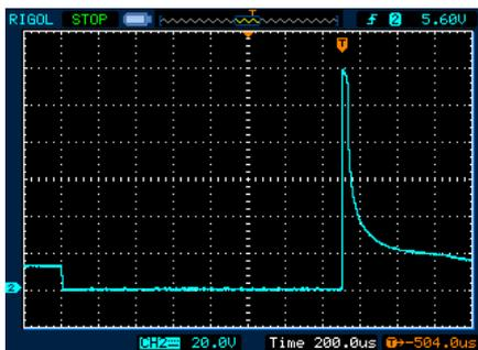
The problem- unprotected injector shows a 120V spike that can damage circuitry. If we completely eliminate the spike the injector is slow to turn off as the current circulates through the protection diode.
