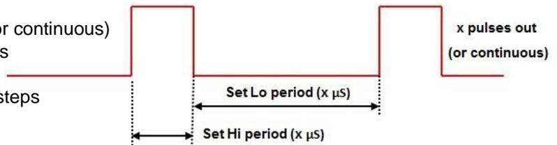
Pulser has an auxiliary input (see Pulser manual) that can remotely start/reset the output pulse counter and this is ideal for designing an injector tester where a set number of pulses each test is the norm.
