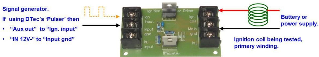
To explore supply voltage relationship to coil current use a variable power supply for the coil.
