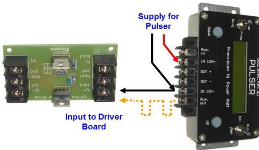
**NOTE:** Although the 'input ground' and 'main ground' are physical joined on the Driver Board circuit, the 'input ground' is not rated for high current. For best performance make sure the 'main ground' terminal is wired to the power supply source for the item under test.
