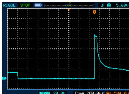
The solution- active clamping of the injector voltage spike protects the circuitry and closely mimics an ECU's behavior. This means that the injector response times match the vehicles when dynamic flow testing.
