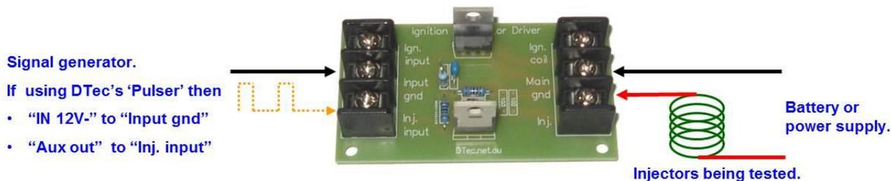
**NOTE:** More than one injector can be wired in parallel (up to 17 Amps). If the MOSFET becomes too hot to touch then fit a heatsink or reduce injectors.
