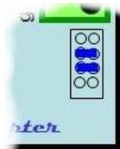
Shown here is the default setting that produces a 2ms (millisecond, 2/1000 second) output pulse when an input is received.
