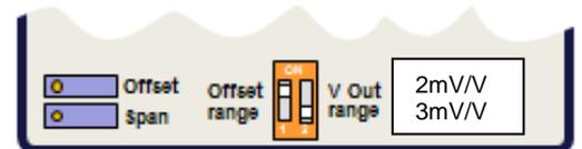
**Span-** Changes the amount of 'gain' (or 'multiplication') that the amplifier has i.e. how much voltage it gives out for a certain input from the load cell.
