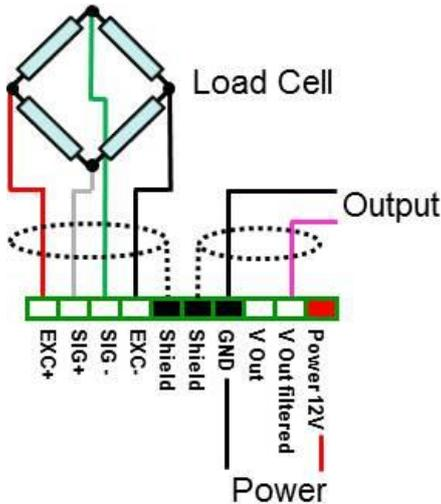
**NOTE:** Connected correctly the output voltage should rise as you apply force in the appropriate direction to the load cell. If the output decreases then reverse either the excitation wires or the signal wires from the load cell!
