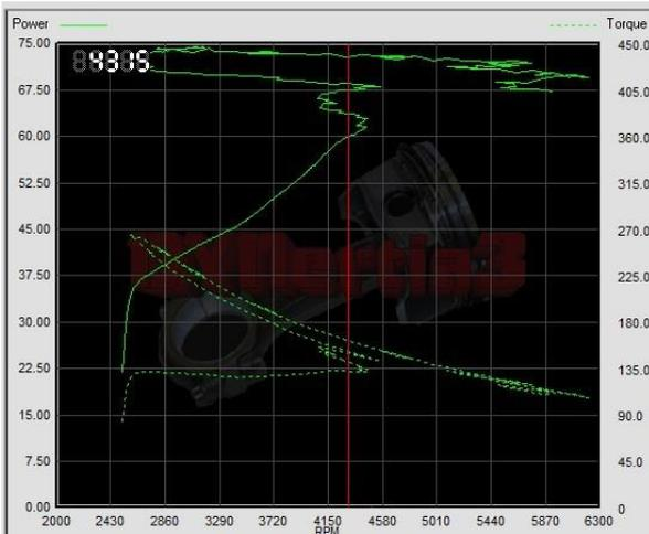
**NOT OK**- Traces go back and forth. This can be from ignition interference etc. but the image above is lacking any large 'spikes' that this usually creates.
