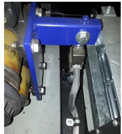
If we know the force (in Nm allowing for the length of 'torque arm') applied to the load cell and the RPM of the shaft we can calculate power by the metric formula  $Kw = (Nm \times RPM) / 9549$ , this will be power at the wheels. By using a chassis dyno we can have a very convenient and quick way of testing modifications, unfortunately the effect of drivetrain losses and tire losses do have an impact.
