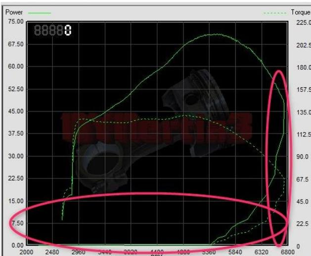
**NOT OK-** Both these traces are running back under themselves at the test end. The trace should not run back under itself or you effectively end up with 2 power readings for every RPM point and this is confusing to calculations we run.
