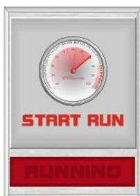
Drive in the test gear (4<sup>th</sup> in this example), hold the speed below what you have set for a 'Run Minimum' with the throttle wide open by using your brake load control.
