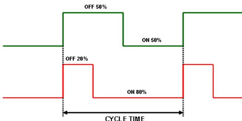
Imagine these signals are operating a switch at high speed to turn on a device. The frequency shown with both has remained the same (they have the same cycle time). What has changed is the amount of that time that has been spent ON compared to OFF (known as 'duty cycle').
