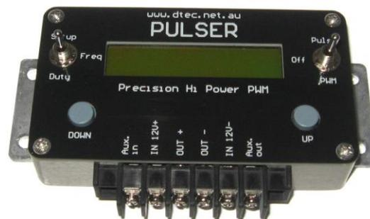
Pulser can also produce pulses of a programmable Hi/Lo duration and count out a set number of these. It can also be triggered and reset from a remote button if desired. This makes it perfect for testing/calibrating injectors or ignition systems. It can easily form part of the testing equipment for such tasks as injector flow testing, measuring 'dead time' (voltage dependent delays) or ignition coil testing and dwell time mapping.
