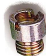
If jets are sized by diameter then we need to calculate the orifice area and use this to approximate the practical flow change. The following formula is simplified from the fact that Area=3.142 x radius<sup>2</sup>.
