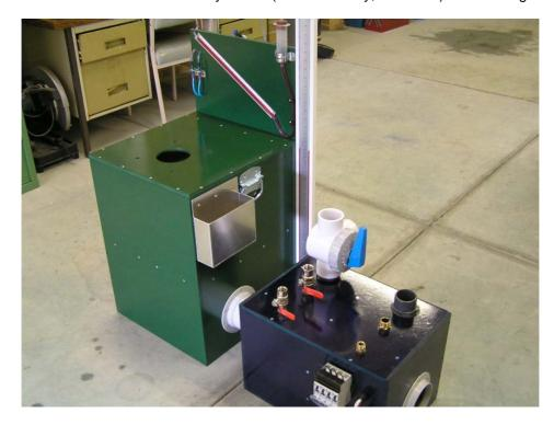
View with the lid removed. Visible is the orifice plate (no 'bungs' fitted in the photo) with captive bolts (bonded in) and wing nuts that allow the orifice plate to be turned over easily for blow testing of exhaust systems etc. Upper pressure sensing tube can be seen on the back wall, there is one below the orifice plate also, their ends are blocked and they have small holes along them (not visible). The wooden blocks on the back wall are what the laminar flow grid rests on.
