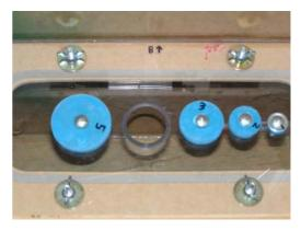
After experimenting unsuccessfully with machining and stamping of very thin gauge plates, the current orifice construction concept was reached. The holes are milled into a Perspex sheet and a steeply angled edge ensures that the edge is very sharp.
