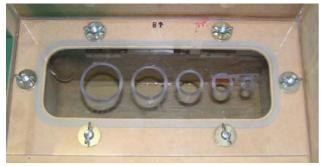
The edges must be angled steeply so that a sharp edge is formed and air does not 'follow' the tapper and become turbulent. The direction of air flow when measuring must be with the air flow hitting the flat side (taper down stream). The whole plate is simply inverted for blow testing. This design behaves as a true 'sharp edge', this was confirmed by testing on a superflow SF-1020 bench at all reasonable pressures.
