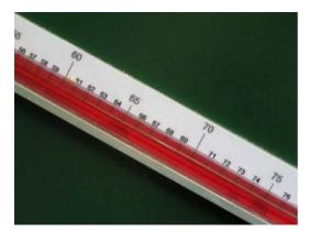
The pressure drop across an orifice is to the square of the flow. If flow doubles, pressure goes up 4 times, therefore the scale on the inclined manometer must follow this non-linear rule, the scale is logarithmic. 0% is at marked at the top with 100% at the bottom end and as you approach 100% the scale should be greatly expanded so that each % reading is a widely spaced graduation.
